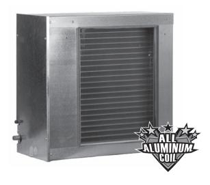
The Amana® brand CSCF Horizontal Slab Evaporator Coils are made for split system air conditioners and heat pumps. This unit features a check flowrater expansion device and rust-resistant, high-temperature, thermoplastic drain pan. Each coil's cabinet has a quality, galvanized-steel finish.
