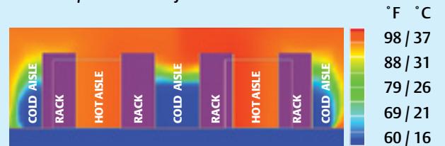
Heat Load = 6 kW Per Rack With Hot Aisle /Cold Aisle Layout
