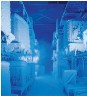
UL testing mandates that coils undergo a minimum of 250,000 stress cycles to insure their integrity. During its lifetime, the typical coil will undergo approximately 500,000 cycles. But Trane is anything but typical. To prove its strength and reliability, we tested the Climatuff coil by subjecting it to over 3 million cycles. The Climatuff coil has also proven itself through extreme temperature testing in Trane's Systems Environmental Extreme Testing (SEET) Lab, where
