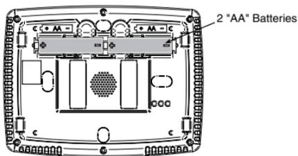
2 "AA" alkaline batteries are included in the control with a battery tag to prevent power drainage. The battery tag must be removed to engage the batteries. The batteries are required to maintain time during a power outage. They are also required for armchair programming.
